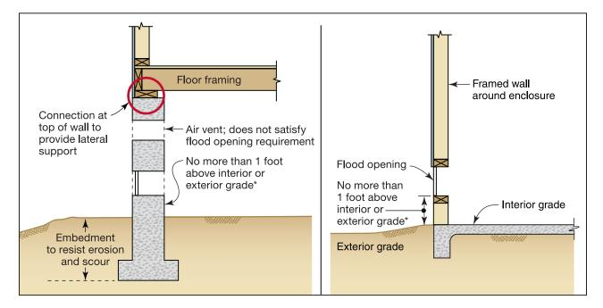
Figure 5E-13. Typical opening for solid foundation wall
